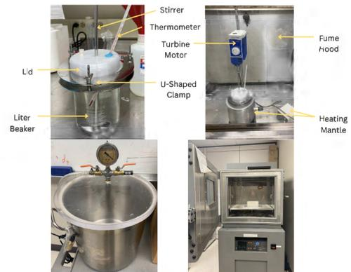
**Figure 1.** The beaker containing the PVA-C mixture after heating (top left). The “cooking” process took place in the fume hood (top right). The Vacuum Chamber with a pressure sensor on top of the lip, it is attached to a motor (bottom left). The Environmental Chamber with a piece of block placed in the center of the chamber (bottom right).
